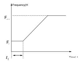
Fig.6-3 Starting frequency and starting time
