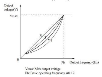
Fig.6-35 Torque-reducing curve
