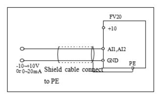
Fig 4-3 Al1, Al2 terminal wiring
