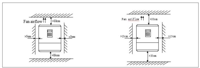
Fig 3-1 Installation interval (Power below 45kW)
