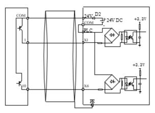
Fig 4-10 Use internal power supply for drain connection
