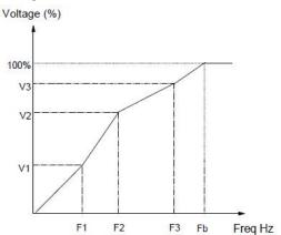
V1~V3: Voltage of sections 1~3 F1~F3: Freq of sections 1~3
