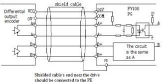
Fig 4-17 Wiring of differential output encoder
