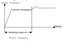
Fig.6-45 Preset frequency of close-loop operation
