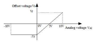
Fig.6-38 Offset of output voltage
