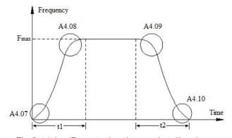
Fig.6-14 Acc/Dec starting time and ending time
