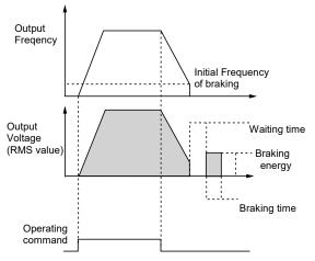
Fig.6-5 Dec-to-stop + DC injection braking
