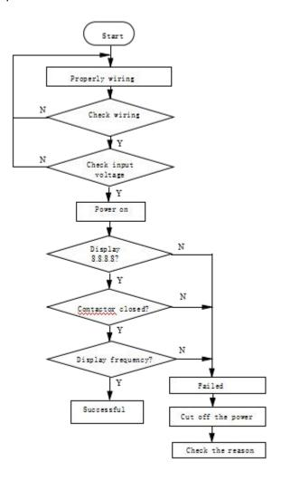
Fig.5-5 Procedures of first-time start-up
