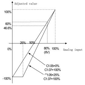
Fig.6-43 Regulation curve of reference
