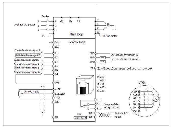
Fig.4-1 Basic wiring chart
