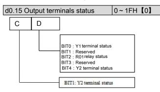
Fig.6-49 Output terminal status
