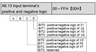
Fig.6-24 terminal's positive and negative logic
