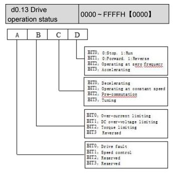
Fig.6-47 The drive's operation status
