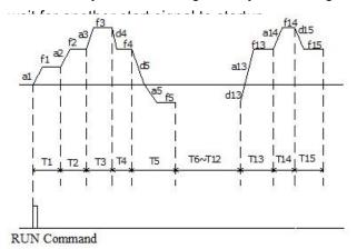
Fig.6-47 Stop after single cycle
