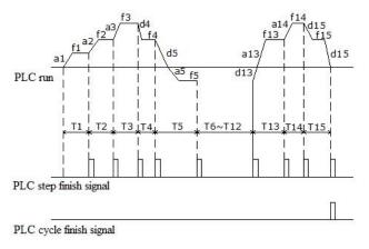
Fig.6-46 Simple PLC function
