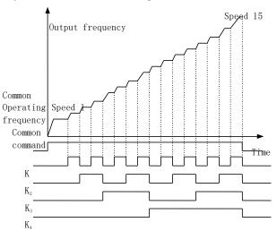
Fig.6-18 Multi-step speed operation
