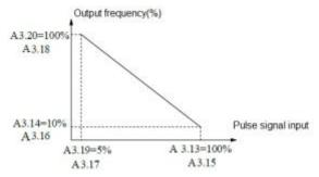
Fig.6-11 Pulse signal input 2
