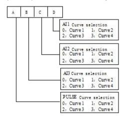
Fig.6-9 Frequency curve selection
