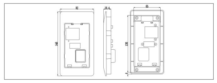
Fig 2-5 Installation box dimension
