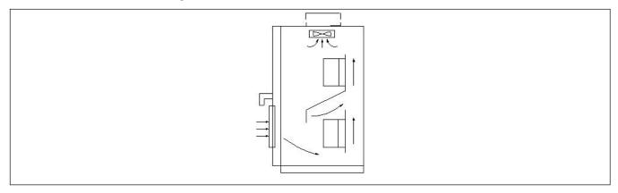
Fig 3-3 Installation of several VFD
