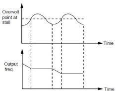
Fig.6-39 Over-voltage at stall
