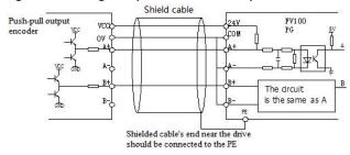
Fig.4-19 Wiring of push-pull output encoder
