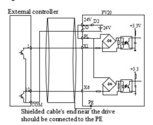
Fig.4-9 Use internal power supply for Source connection
