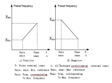
Fig.6-8 Freq. corresponding to Min. frequency
