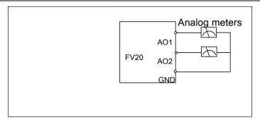
Fig.4-4 Wiring of analog output
