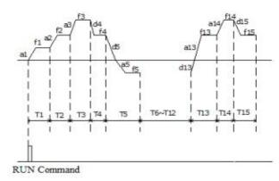
Fig.6-48 Keep final states after single cycle
