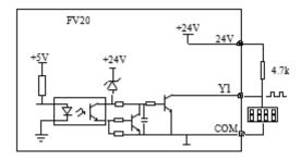
Fig 4-15 Wiring method 1 of output terminal Y2
