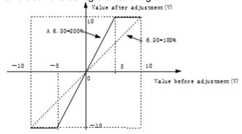
Fig.6-31 Relationship curve between analog output and gain
