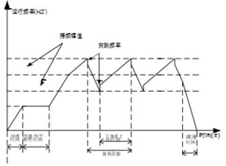
Fig. 6-56Schematic diagram of swing frequency
