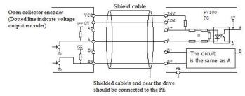
Fig.4-18 Wiring of open collector output encoder
