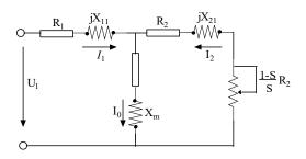
Fig. 6-33 Motor's equivalent circuit
