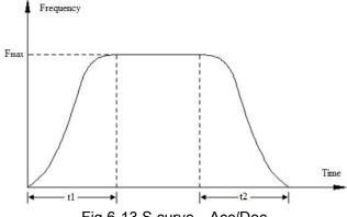
S curve Acc/Dec mode can smooth acceleration and deceleration, suitable for application like lift, conveyer belt.
