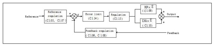
Fig.6-41 Principle diagram of process close-loop control
