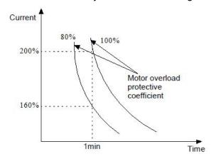
Fig.6-34 Motor's overload protection coefficient
