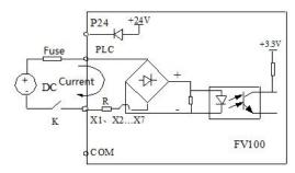
Fig.4-8 Wiring of external power supply
